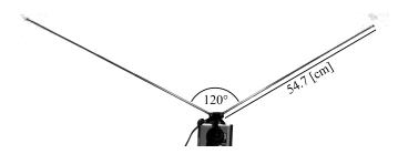
Fig. 1. Dipole antenna dimensions
