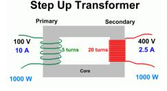
Fig. 2. Step up transformer (3)
