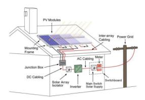
Fig. 3. Model of domestic grid-enabled solar system (4)
