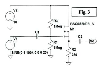
21. (4 pts) What is the closest minimum value of C1 that will both block dc and provide low loss (no more than -3dB attenuation) at 100kHz?
