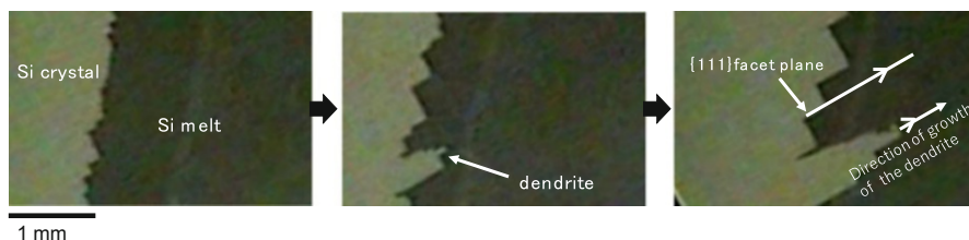
Fig. 7 Dendrite growth initiated from a part of zigzag faceted interface (Fujiwara et al. 2007)
