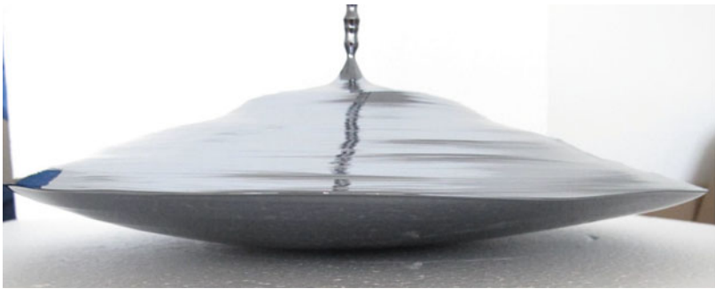
p -Type single ingot (NOC-6) with a convex growth interface grown after furnace cleaning. Maximum diameter: 35.0 cm Diameter ratio: 0.7 Height: 8.0 cm
