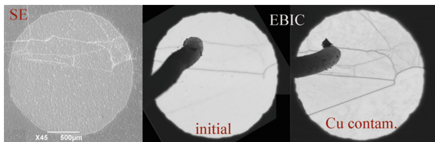
Fig. 16 EBIC images of mc-Si before and after Cu diffusion. The SE image is shown in the left image
