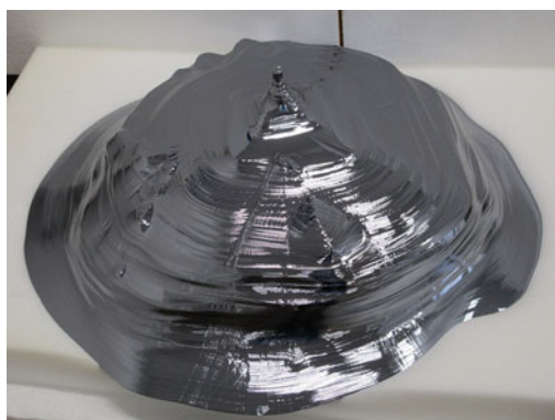
Fig. 14 Si multicrystalline ingot with some dendrite crystals. The dendrite crystals appeared in front of the growth interface during growth owing to the local temperature fluctuation of larger than 10 K.
