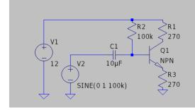
Fig. 3. Common Emitter Amplifier Schematic
