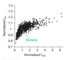
FIGURE 7.24 Ion vs. Ioff with variation
