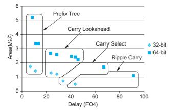
FIGURE 11.40 Area vs. delay of synthesized adders
