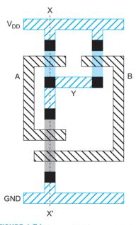
FIGURE 1.74 2-input NAND gate stick diagram
