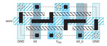
FIGURE 12.15 Lithographically friendly 6T SRAM cell
