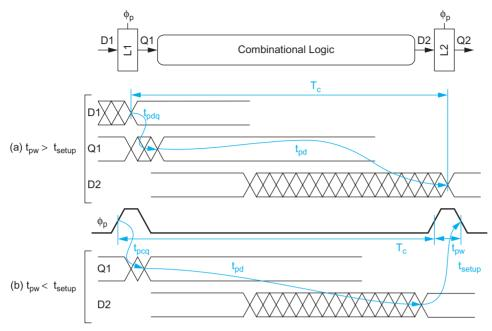
FIGURE 10.8 Pulsed latch max-delay constraint
