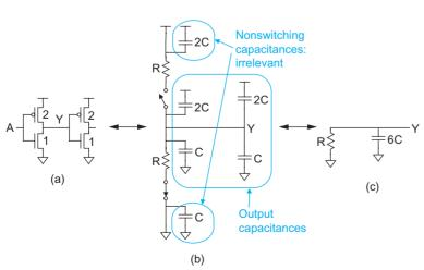
FIGURE 4.6 Equivalent circuit for an inverter
