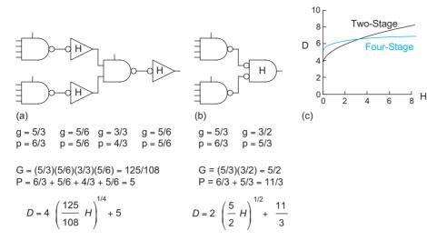
FIGURE 9.43 8-input domino AND delays
