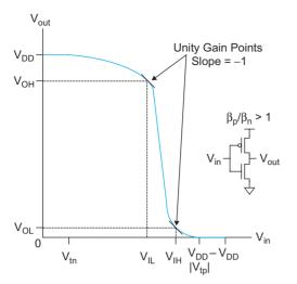
FIGURE 2.30 CMOS inverter noise margins
