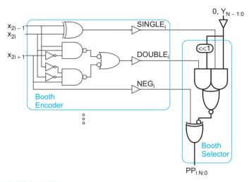
FIGURE 11.80 Radix-4 Booth encoder and selector
