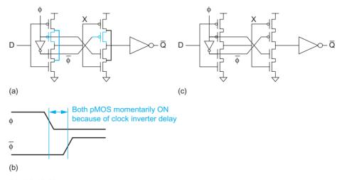
FIGURE 10.20 Transmission gate and NORA dynamic flip-flops
