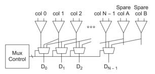
FIGURE 12.81 Column redundancy
