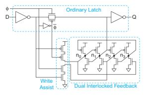
FIGURE 10.32 Radiation-hardened latch
