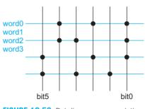
FIGURE 12.53 Dot diagram representation of ROM
