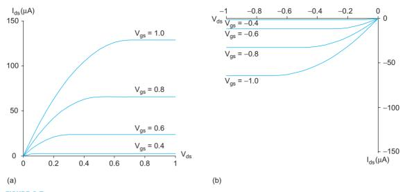
FIGURE 2.7 I-V characteristics of ideal 4/2  $\lambda$  (a) nMOS and (b) pMOS transistors
