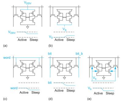
FIGURE 12.37 Leakage reduction techniques
