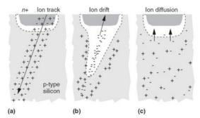
FIGURE 7.11 Generation and collection of carriers after a radiation strike (© IEEE 2005.)
