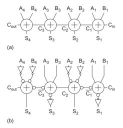
FIGURE 11.11 4-bit carry-ripple adder
