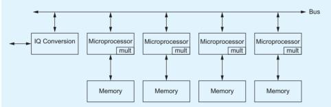
FIGURE 14.11 Enhanced multiprocessor for software radio
