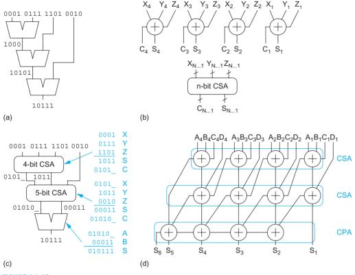
FIGURE 11.42 Multiple-input adders
