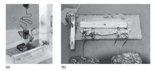
FIGURE 1.2 (a) First transistor (Property of AT&T Archives. Reprinted with permission of AT&T.) and (b) first integrated circuit (Courtesy of Texas Instruments.)
