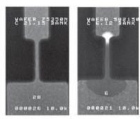
Intact Blown FIGURE 3.30 eFUSE (© IEEE 2005.)
