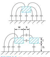
**FIGURE 6.9** Effect of fringing fields on capacitance
