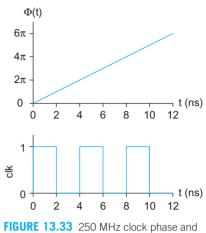
FIGURE 13.33 250 MHz clock phase and waveform
