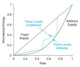
FIGURE 5.18 Energy reduction from DVS
