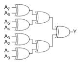
FIGURE 11.57 8-bit parity generator
