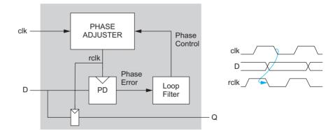
FIGURE 13.74 Phase calibration loop for mesochronous timing recovery
