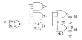
FIGURE 4.32 Example path annotated with transistor sizes
