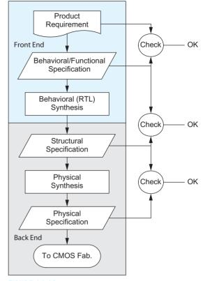
FIGURE 14.19 Generalized design flow
