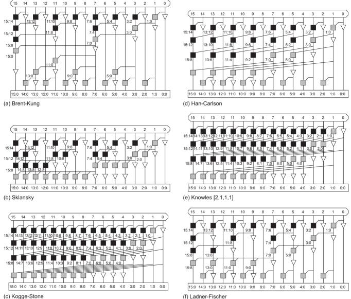
FIGURE 11.29 Tree adder PG networks
