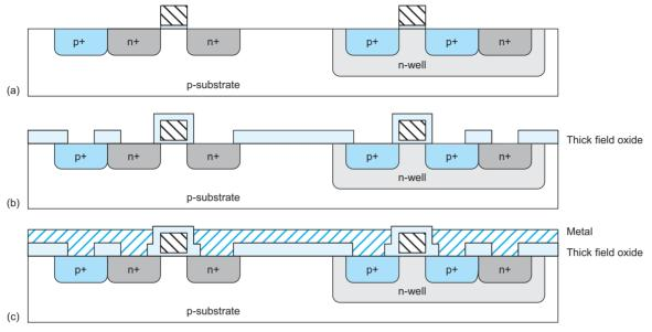
FIGURE 1.38 Cross-sections while manufacturing p-diffusion, contacts, and metal
