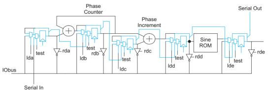
FIGURE 14.21 Scan register insertion for testing
