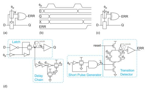
FIGURE 10.41 Adaptive sequencing elements
