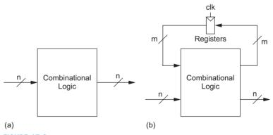
FIGURE 15.6 The combinational explosion in test vectors
