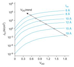
FIGURE 2.21 Gate leakage current from [Song01]
