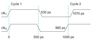
FIGURE 13.19 Skewed clock waveforms
