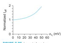
FIGURE 7.26 Impact of random threshold voltage on average leakage
