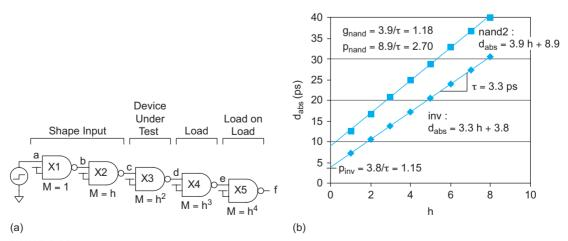
FIGURE 8.30 Logical effort characterization of 2-input NAND gate and inverter
