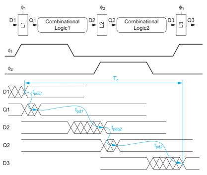
FIGURE 10.7 Two-phase latch max-delay constraint
