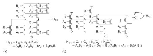
FIGURE 11.37 3-bit and 4-bit pseudogenerate gates using primary inputs
