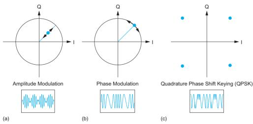
FIGURE 14.4 Examples of IQ modulation
