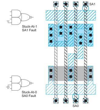
FIGURE 15.11 CMOS stuck-at faults
