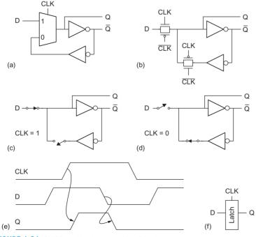
FIGURE 1.31 CMOS positive-level-sensitive D latch
