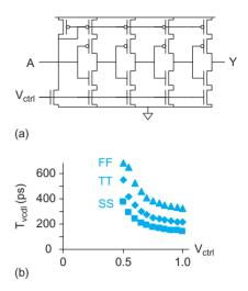
FIGURE 13.42 An example of a voltagecontrolled delay line (VCDL) (a) a currentstarved inverter chain, (b) its voltage-to-delay characteristics for various process conditions
