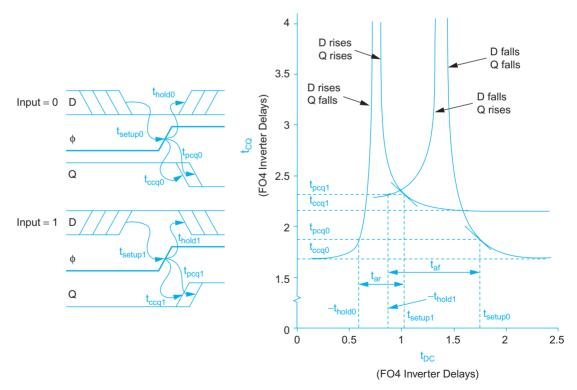
FIGURE 10.36 Flip-flop setup and hold times
