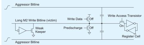
FIGURE 15.25 Register file write circuitry
