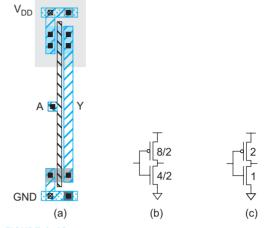
FIGURE 1.40 Inverter with dimensions labeled
