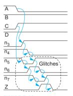
FIGURE 5.10 Glitching in a chain of gates
