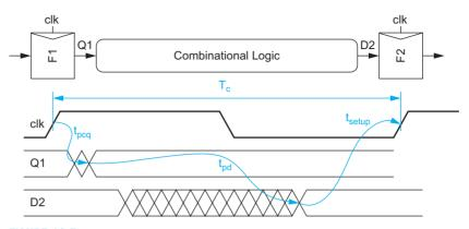
FIGURE 10.5 Flip-flop max-delay constraint
