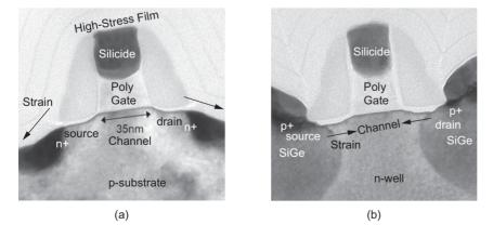
FIGURE 3.19 Strained silicon transistor micrographs: (a) nMOS, (b) pMOS (© IEEE 2005.)
