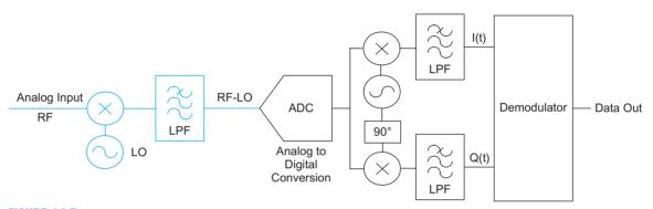
FIGURE 14.5 Software radio receive path
