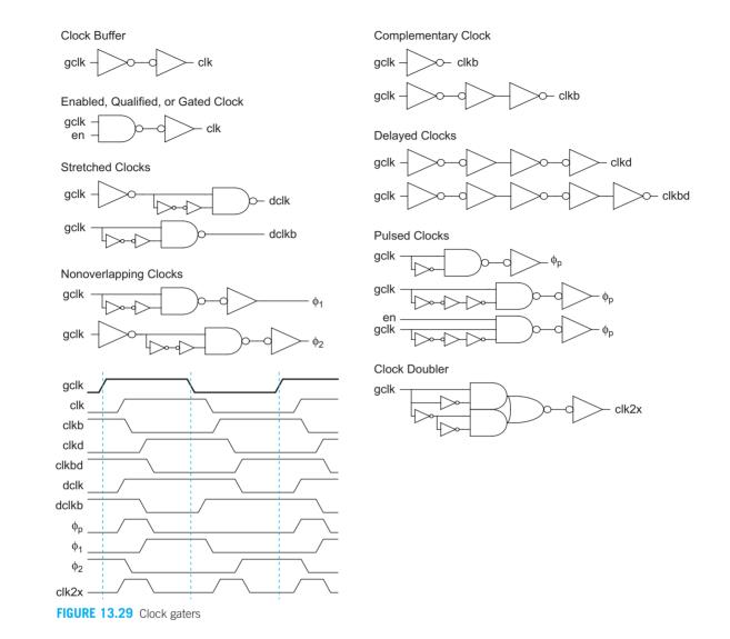
short as possible. Variations in the input threshold of the clocked elements also causes skew. The best way to limit this skew is to produce crisp rise/fall times at the clock gaters. The final stage should have a fanout of no more than about 4.
