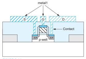
FIGURE 3.11 Aluminum metallization
