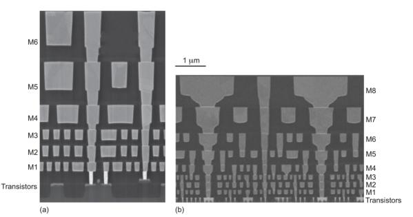
**FIGURE 6.2** SEM image of wire cross-sections in Intel's (a) 90 nm and (b) 45 nm processes ((a) From [Thompson02] © 2002 IEEE. (b) From [Moon08] with permission of Intel Corporation.)
