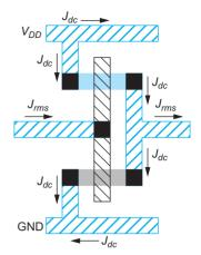
FIGURE 7.10 Current density limits in an inverter
