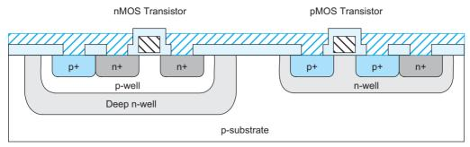
FIGURE 3.5 Well structure in triple-well process
