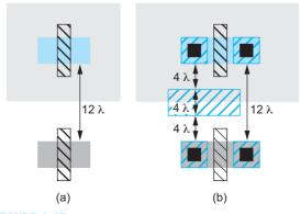
FIGURE 1.45 Spacing between nMOS and pMOS transistors
