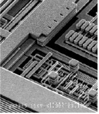
FIGURE 3.13 Cross-section showing 11 levels of metallization (Courtesy of International Business Machines Corporation. Unauthorized use not permitted.)
