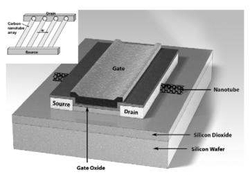
FIGURE 3.35 Carbon nanotube transistor (© IEEE 2003.)
