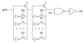
FIGURE 13.32 Digitally adjustable delay line
