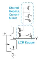
FIGURE 9.38 Leakage current replica keeper
