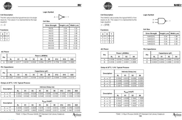
Figure 4.25 Artisan Components cell library datasheets. Reprinted with permission.
