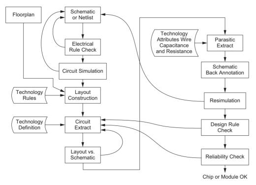
FIGURE 14.25 Mixed-signal or custom-design flow
