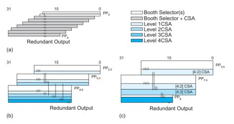
FIGURE 11.91 16 × 16 Booth-encoded multiplier floorplans: (a) array, (b) Wallace tree, (c) [4:2] tree
