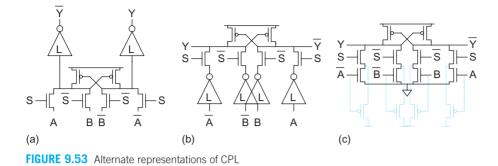
include the inverters from the previous stage that drives the diffusion input, but to exclude the output inverters. Figure 9.53(c) shows the mux drawn at the transistor level. Observe that this is identical to the CVSL gate from Figure 9.47 except that the internal node of the stack can be pulled up through the weak pMOS transistors in the inverters.
