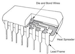
FIGURE 13.2 Cutaway view of dual-in-line package (© IEEE 1985.)
