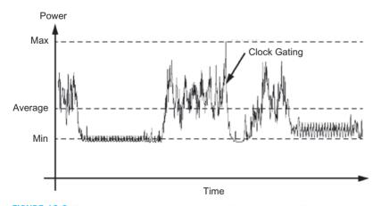
**FIGURE 13.6** Time-dependent power consumption of microprocessor (Reprinted with permission of Sun Microsystems.)
