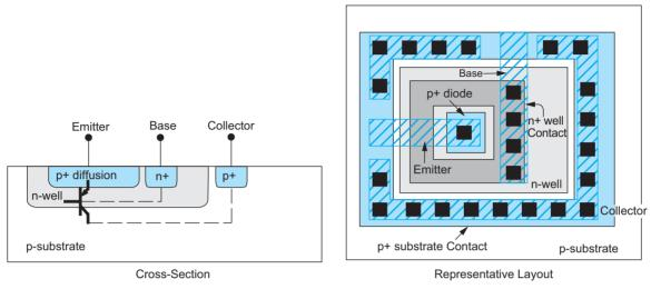
FIGURE 3.27 Vertical pnp bipolar transistor
