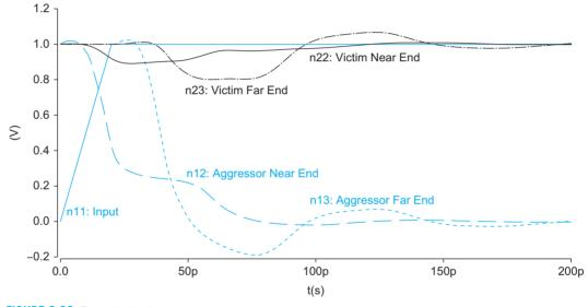
FIGURE 8.36 Transmission line response
