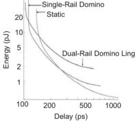
**FIGURE 11.38** Energy-delay trade-offs for 90 nm 32-bit Sklansky static, domino, and dual-rail domino adders. FO4 inverter delay in this process at 1.0 V and nominal  $V_t$  is 31 ps. (© IEEE 2007.)
