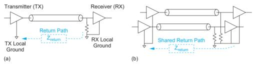
FIGURE 13.60 Simultaneous switching noise mechanism (a) ISI, (b) crosstalk
