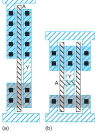
**FIGURE 4.18** Layout styles: (a) conventional, (b) folded
