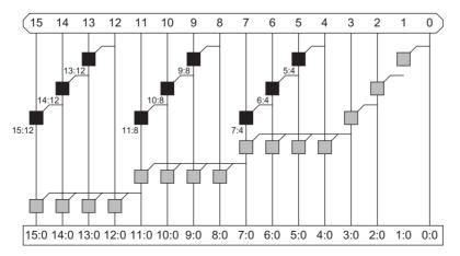
FIGURE 11.25 Carry-increment adder PG network
