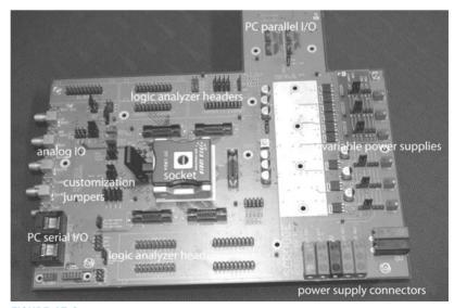
FIGURE 15.2 Typical test board
