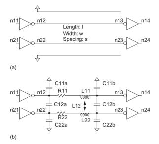
FIGURE 8.33 Lossy multiconductor transmission lines
