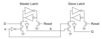
FIGURE 10.45 Fast synchronizer flip-flop
