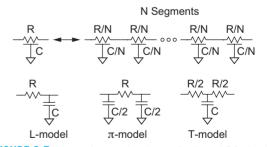
FIGURE 6.5 Lumped approximation to distributed RC circuit
