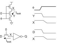
FIGURE 9.65 Pass gate leakage in dynamic latches and gates
