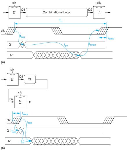
FIGURE 10.15 Clock skew and flip-flops
