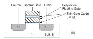
FIGURE 12.57 Cross-section of floating gate nMOS transistor
