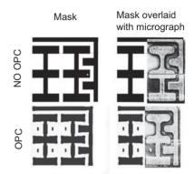
FIGURE 3.4 Subwavelength features printed with and without OPC. Predistortion of corners in OPC reduces undesired rounding. (Adapted from [Schellenberg98] with permission of SPIE.)
