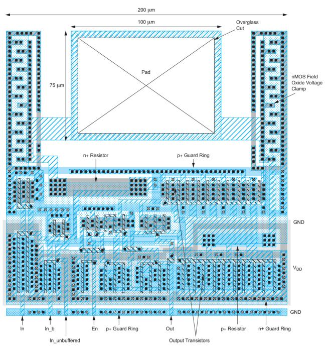
**FIGURE 13.51** MOSIS 1.6  $\mu$ m bidirectional pad. Color version on inside front cover.
