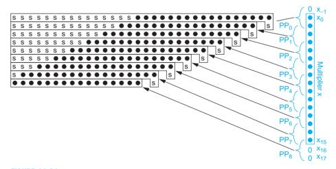
FIGURE 11.81 Radix-4 Booth-encoded partial products with sign extension
