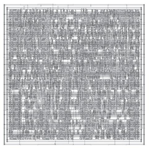
FIGURE 1.65 Synthesized MIPS processor
