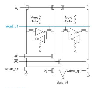
FIGURE 12.31 Complete pair of columns for two-way multiplexed SRAM
