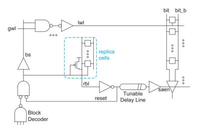
FIGURE 12.30 Replica delay for sense amplifier enable
