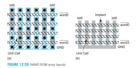
ROMs are often broken into multiple small banks with a limited number of series transistors. Nevertheless, these NAND structures are attractive for Flash memories in which density and cost are more important than access time.
