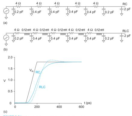
FIGURE 6.21 Wide clock line modeled with and without inductance
