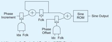
(a) Numerically Controlled Oscillator (NCO) Structure
