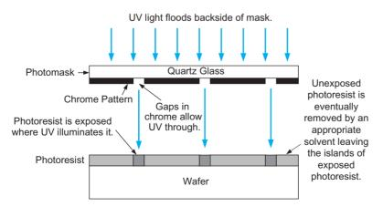
**FIGURE 3.3** Photomasking with a negative resist (lens system between mask and wafer omitted to improve clarity and avoid diffracting the reader <sup>(C)</sup>)
