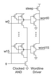
FIGURE 12.21 Shared clock and transistors in wordline driver
