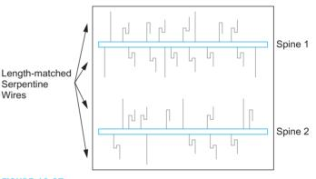
FIGURE 13.27 Clock spines with serpentine routing
