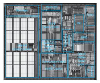
FIGURE 7.35 Pentium III microprocessor (Courtesy of Intel Corporation.)
