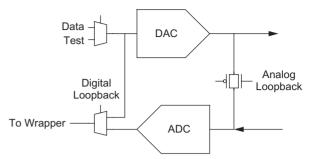
FIGURE 15.21 Analog and digital loopback
