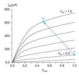
FIGURE 4.20 Approximate switching trajectory
