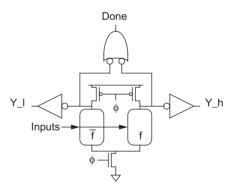
FIGURE 9.31 Dual-rail domino gate with completion detection
