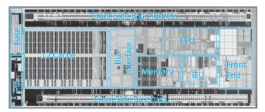
FIGURE 7.38 Atom Processor (Courtesy of Intel Corporation.)
