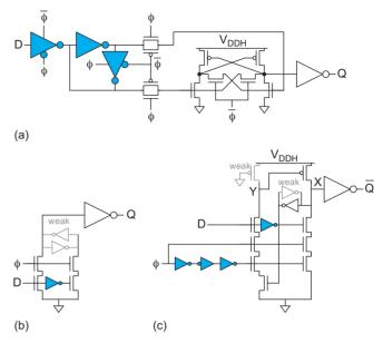
FIGURE 10.40 Level-converter flip-flops and latches
