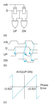
FIGURE 13.75 Hogge detector (a) circuit, (b) waveforms, (c) transfer curve
