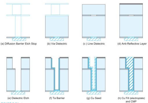
FIGURE 3.21 Copper dual damascene interconnect processing steps
