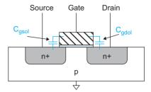
FIGURE 2.10 Overlap capacitance
