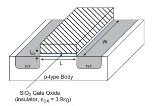
FIGURE 2.6 Transistor dimensions
