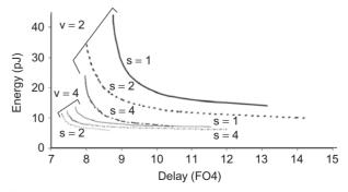
**FIGURE 11.39** Energy-delay trade-offs for 90 nm 64-bit domino Kogge-Stone Ling adders as a function of valency (*v*) and sparseness (*s*). (© IEEE 2009.)
