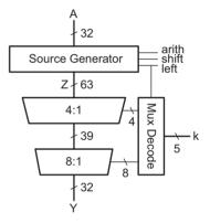
FIGURE 11.65 32-bit logarithmic funnel shifter
