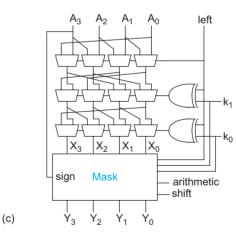
FIGURE 11.68 Barrel shifters: (a) rotate right, (b) rotate left or right, (c) rotates and shifts
