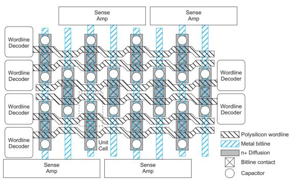
FIGURE 12.46 Layout of folded bitline subarray
