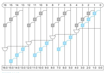
FIGURE 11.18 Carry-skip adder PG network
