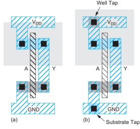
FIGURE 1.41 Inverter cell layout
