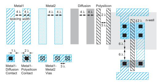
**FIGURE 1.39** Simplified  $\lambda$ -based design rules
