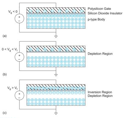
FIGURE 2.2 MOS structure demonstrating (a) accumulation, (b) depletion, and (c) inversion
