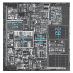
FIGURE 7.36 Pentium III microprocessor (Courtesy of Intel Corporation.)
