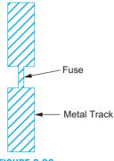
FIGURE 3.29 A typical metal fuse
