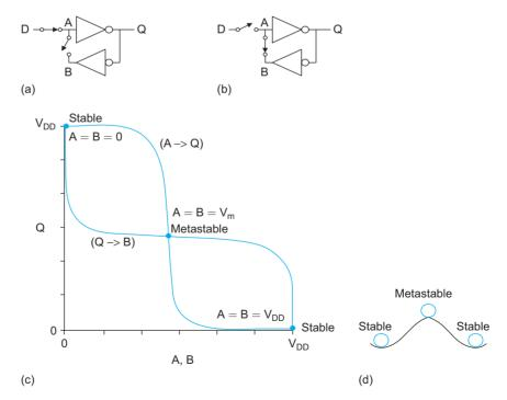
FIGURE 10.42 Metastable state in static latch
