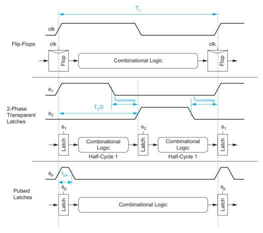
FIGURE 10.2 Static sequencing methods
