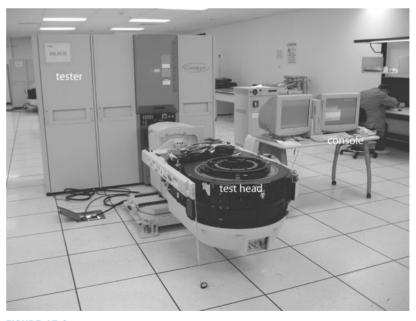
FIGURE 15.3 The Teradyne Catalyst: A typical production tester (Photo: John Haddy, Cisco Systems.)
