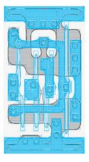
FIGURE 7.21 Discrepancy between drawn and printed layout of NAND gate caused by subwavelength lithography (© 2007 Larry Pileggi, reprinted with permission.)
