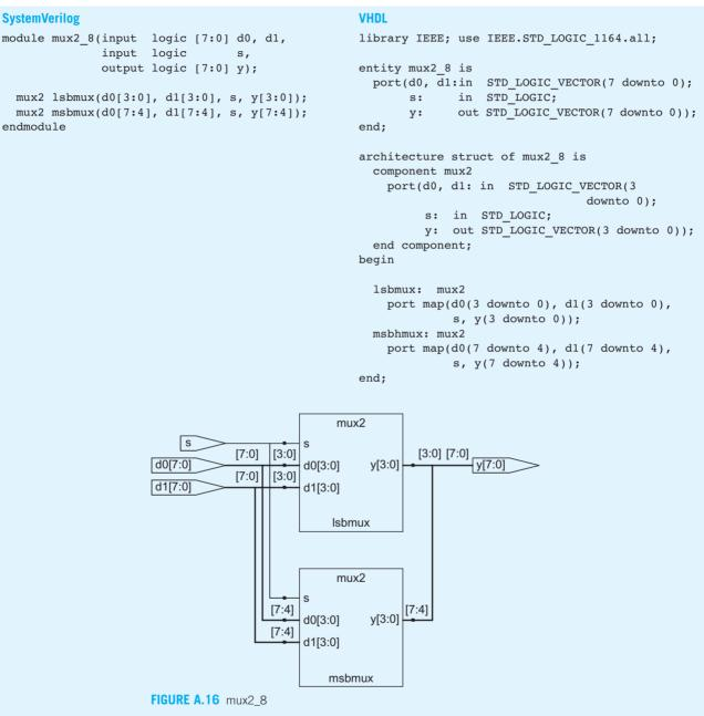
In general, complex systems are designed *hierarchically*. The overall system is described structurally by instantiating its major components. Each of these components is described structurally from its building blocks, and so forth recursively until the pieces are simple enough to describe behaviorally. It is good style to avoid (or at least minimize) mixing structural and behavioral descriptions within a single module.
