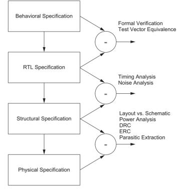
FIGURE 15.1 Functional equivalence at various levels of abstraction
