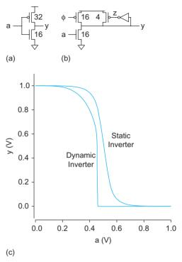
FIGURE 8.28 Circuits for DC transfer analysis
