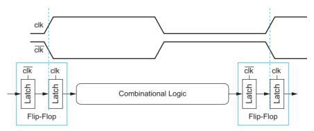
FIGURE 10.3 Flip-flop viewed as back-to-back latch pair
