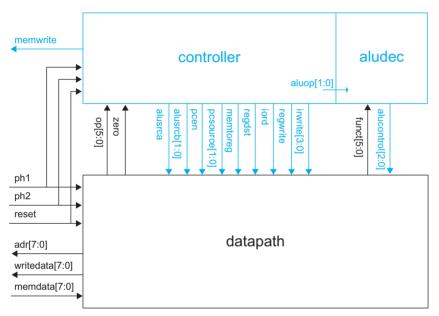
FIGURE 1.56 Top-level MIPS block diagram
