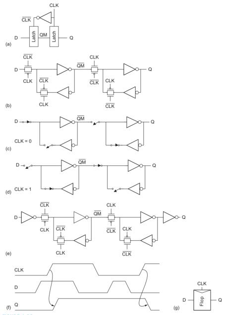
FIGURE 1.32 CMOS positive-edge-triggered D flip-flop
