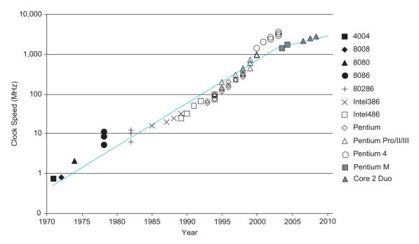
FIGURE 1.5 Clock frequencies of Intel microprocessors
