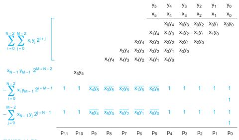
FIGURE 11.76 Partial products for two's complement multiplier
