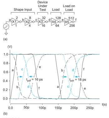
FIGURE 8.9 Fanout-of-4 inverters
