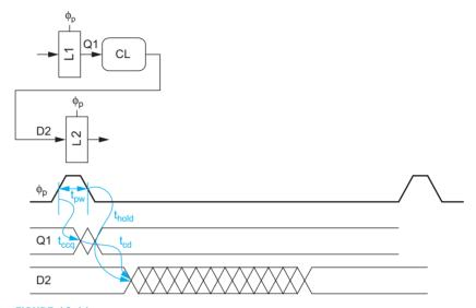
FIGURE 10.11 Pulsed latch min-delay constraint
