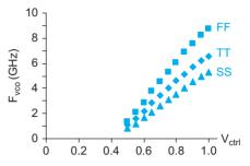
FIGURE 13.36 VCO voltage-to-frequency characteristics over different process conditions
