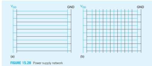
Modern chips require low-resistance on-chip power distribution networks and often use power and ground pads distributed across the die rather than just at the periphery to reduce the distance and resistance between the pads and the gates. Power integrity analysis should be performed to verify that the static or dynamic voltage droops remain within their budget everywhere on the chip.
