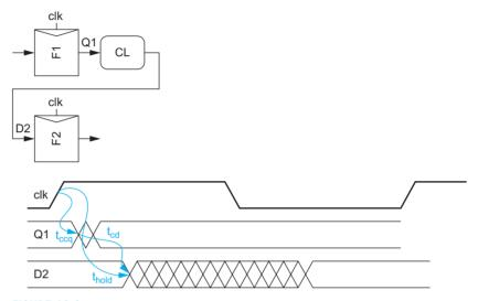
FIGURE 10.9 Flip-flop latch min-delay constraint
