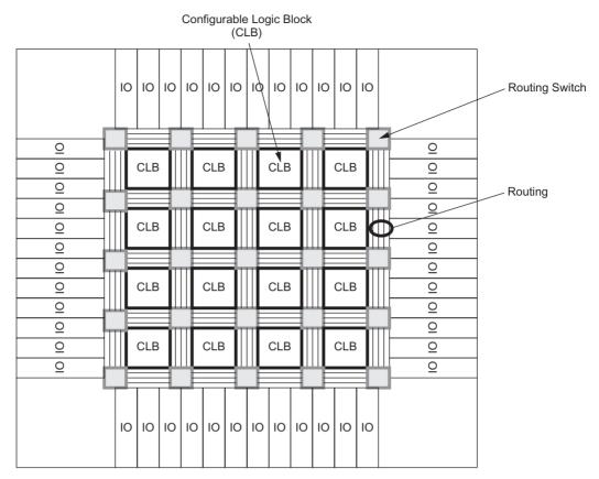
FIGURE14.15 Simplified FPGA floorplan
