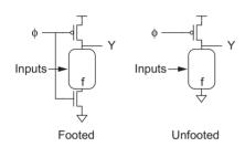
FIGURE 9.24 Generalized footed and unfooted dynamic gates
