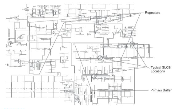
FIGURE 13.25 Itanium 2 modified H-tree
