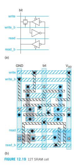
The trade-off between read margin, write margin, transistor sizes, and operating voltage limits the minimum operating voltage of a compact 6T cell. Using an 8T dual-port cell for single-ported operation circumvents these trade-offs and allows lower-voltage operation [Chang08]. Intel switched from 6T to 8T cells within the cores for its 45 nm line of Core processors [Kumar09].
