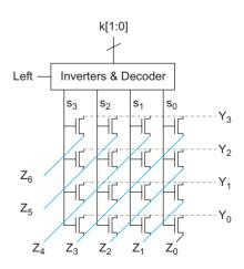
FIGURE 11.62 4-bit array funnel shifter
