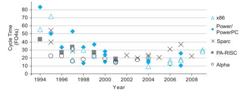
FIGURE 4.38 Microprocessor cylcle time trends. Data has some uncertainty based on estimating FO4 delay as a function of feature size.
