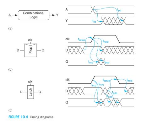
after some *D*-to-*Q* delay  $t_{cdq}$  and  $t_{pdq}$ . Section 10.4.2 discusses how to measure the setup and hold times and propagation delays in simulation.
