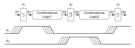
FIGURE 10.16 Clock skew and transparent latches
