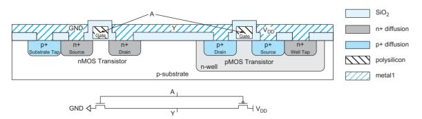
FIGURE 1.34 Inverter cross-section with well and substrate contacts. Color version on inside front cover.
