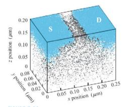
FIGURE 7.23 Random placement of dopant atoms in a 50 nm process. Adapted from [Bernstein06]. (Courtesy of International Business Machines Corporation. Unauthorized use not permitted.)
