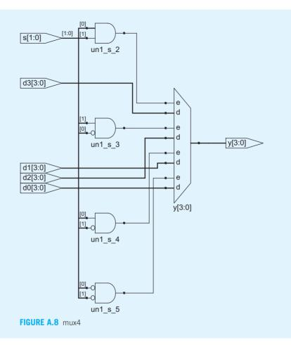
Figure A.8 shows the schematic for the 4:1 multiplexer produced by Synplify Pro. The software uses a different multiplexer symbol than this text has shown so far. The multiplexer has multiple data (d) and one-hot enable (e) inputs. When one of the enables is asserted, the associated data is passed to the output. For example, when s[1] = s[0] = 0, the bottom AND gate un1\_s\_5 produces a 1, enabling the bottom input of the multiplexer and causing it to select d0[3:0].
