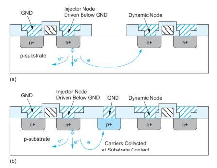
FIGURE 9.58 Minority carrier injection and collection
