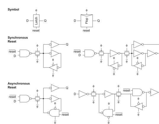
FIGURE 10.24 Resettable latches and flip-flops
