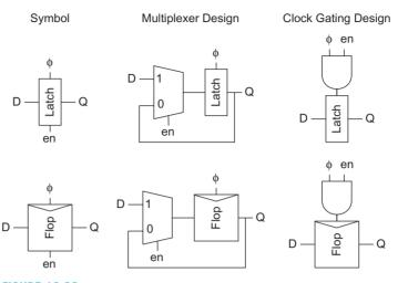
FIGURE 10.26 Enabled latches and flip-flops
