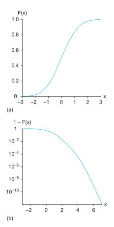
**FIGURE 7.18** Cumulative distribution function for a standard normal random variable
