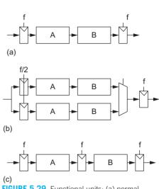
**FIGURE 5.29** Functional units: (a) normal, (b) parallel, (c) pipelined
