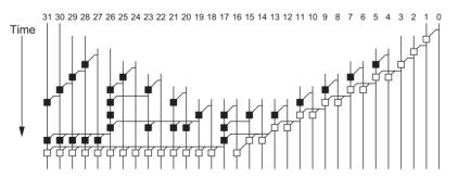
FIGURE 11.94 CPA prefix network with nonuniform input arrival times
