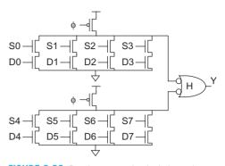
FIGURE 9.29 Domino gate using logic in static CMOS stage
