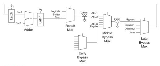
FIGURE 10.14 ALU self-bypass path with two-phase latches
