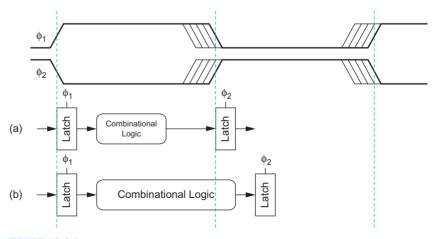
FIGURE 10.34 Latch placement and time borrowing
