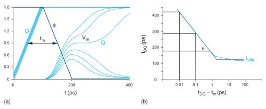
FIGURE 10.43 Metastable transients and propagation delay
