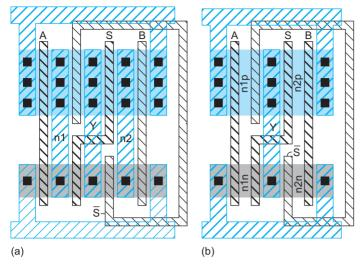
FIGURE 9.50 Multiplexer layout comparison
