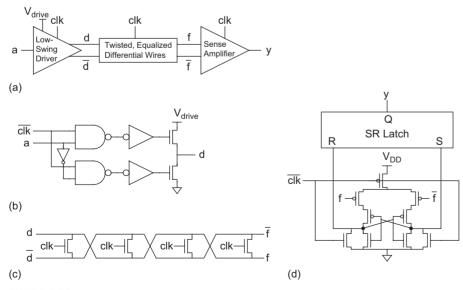
FIGURE 6.30 Low-swing signaling system
