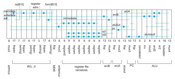
FIGURE 1.68 Datapath slice plan
