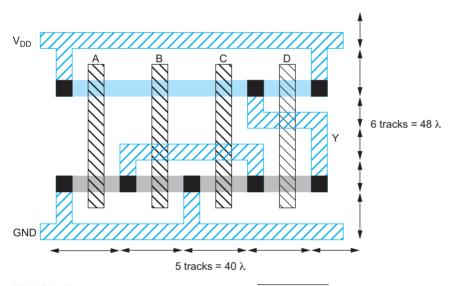
**FIGURE 1.47** CMOS compound gate for function  $Y = (A + B + C) \cdot D$
