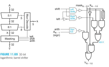
FIGURE 11.70 Barrel shifter masking logic
