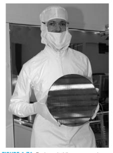
FIGURE 1.71 Engineer holding processed 12-inch wafer (Photograph courtesy of the Intel Corporation.)
