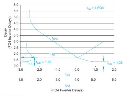
FIGURE 10.37 Latch delay vs. data arrival time
