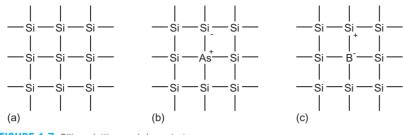
FIGURE 1.7 Silicon lattice and dopant atoms
