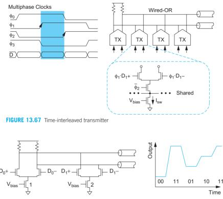
FIGURE 13.68 Multilevel transmitter
