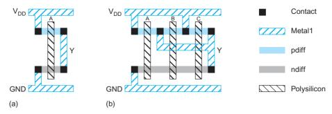
FIGURE 1.43 Stick diagrams of inverter and 3-input NAND gate. Color version on inside front cover.
