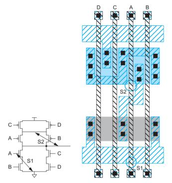
FIGURE 15.12 CMOS bridging faults
