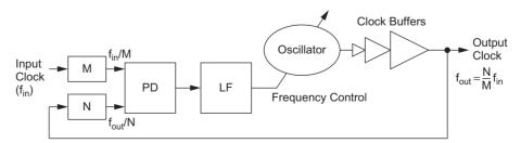
FIGURE 13.23 Frequency multiplication using a PLL
