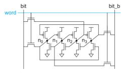
FIGURE 12.82 Radiation-hardened SRAM cell
