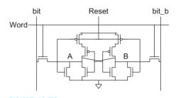
**FIGURE 13.78** Chip identification bit cell
