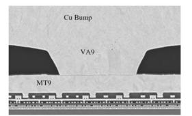
FIGURE 6.3 SEM image of complete cross-section of Intel's 45 nm process including M9 and I/O bump (From [Moon08] with permission of Intel Corporation.)
