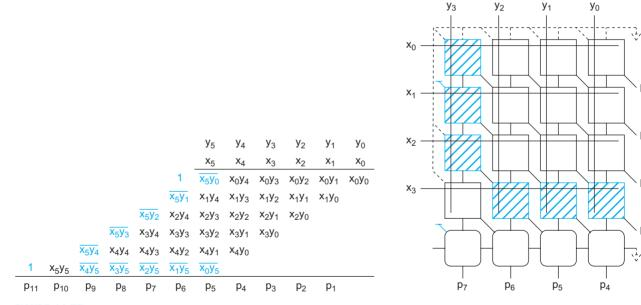
FIGURE 11.77 Simplified partial products for two's complement multiplier
