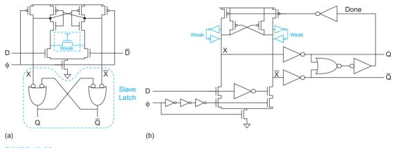
FIGURE 10.29 Differential flip-flops
