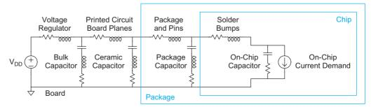
FIGURE 13.10 Power distribution system model
