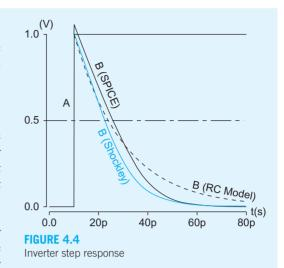
that *B* also initially rises momentarily before falling. This effect is called bootstrapping and will be discussed in Section 4.4.6.6. The dashed black line shows an RC model that approximates the nMOS transistor as a 1 k $\Omega$  resistor when it is ON. The propagation delay predicted by the RC model matches SPICE fairly well, although the fall time is overestimated. RC models will be explored further in Section 4.3.
