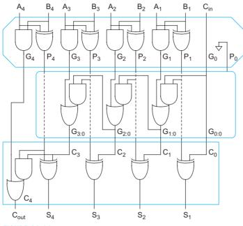
FIGURE 11.14 4-bit carry-ripple adder using PG logic
