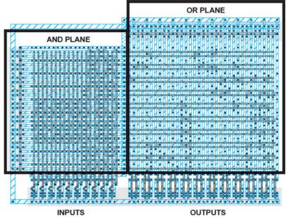
FIGURE 1.69 PLA for control FSM
