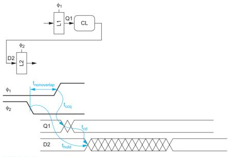
FIGURE 10.10 Two-phase latch min-delay constraint
