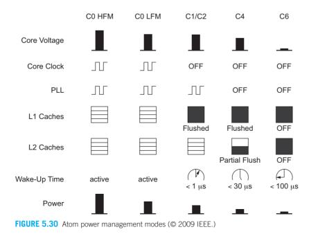
reduces to 0.75 V. In sleep mode C1, the core clock is turned off and the level 1 cache is flushed and power-gated to reduce leakage, but the processor can return to active state in 1 microsecond. In sleep mode C4, the PLL is also turned OFF. In sleep mode C6, the core and caches are all power-gated to reduce power to less than 80 mW, but wake-up time rises to 100 microseconds. For a typical workload, the processor can spend 80–90% of its time in C6 sleep mode, reducing average power to 220 mW.
