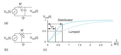
FIGURE 6.24 Lumped and distributed RC circuit response
