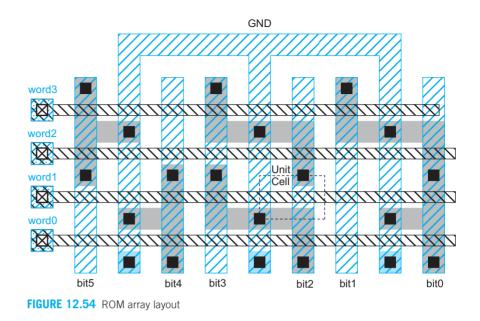
The wordlines run horizontally in polysilicon, while the bitlines and grounds run vertically in metal1. Notice how each ground is shared between a pair of cells. Each bit of the ROM occupies a  $12 \times 8 \lambda$  cell<sup>2</sup>. Polysilicon wordlines are only appropriate for small or slow ROMs. A larger ROM can run metal2 straps over the polysilicon and contact the two periodically (e.g., every eight columns). Occasional substrate contacts are also required.
