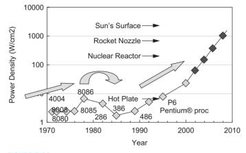
**FIGURE 5.33** Microprocessor power density trends as predicted in 2001 (Reprinted with permission of Intel Corporation.)
