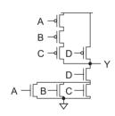
FIGURE 1.19 CMOS compound gate for function  $Y = (\overline{A + B + C}) \cdot \overline{D}$
