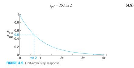
The factor of  $\ln 2 = 0.69$  is cumbersome. The effective resistance *R* is an empirical parameter anyway, so it is preferable to incorporate the factor of  $\ln 2$  to define a new effective resistance  $R' = R \ln 2$ . Now the propagation delay is simply R'C. For the sake of convenience, we usually drop the prime symbols and just write
