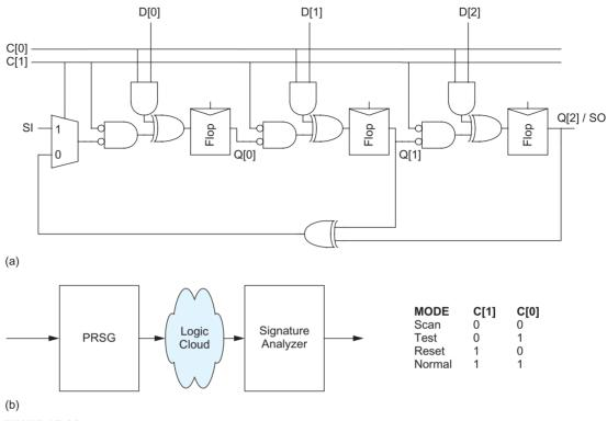
FIGURE 15.20 BIST (a) 3-bit register, (b) use in a system
