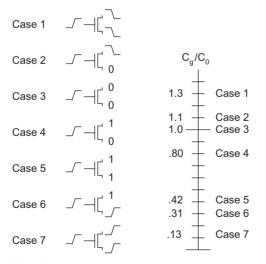
FIGURE 2.11 Data-dependent gate capacitance
