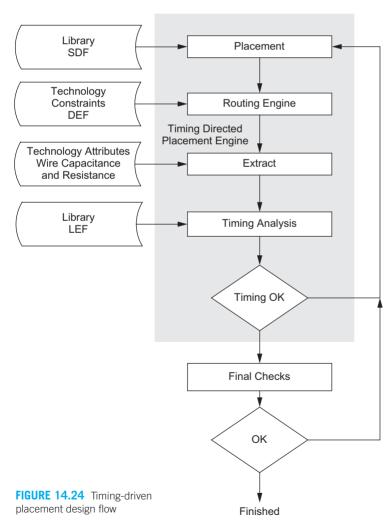
analysis is done to estimate timing. The timing is not known until the physical layout is complete. If timing problems are found, the cycle has to be repeated with some kind of constraint placed on the problematic paths. With complex designs this quickly gets out of control, to the point where changing something on one iteration could undo something fixed on a previous iteration. There are stories of designs that never were completed because of this problem.
