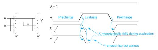
FIGURE 9.27 Incorrect connection of dynamic gates
