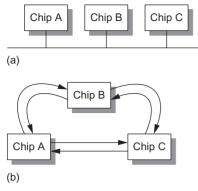
**FIGURE 13.58** (a) multidrop bus vs. (b) point-to-point links
