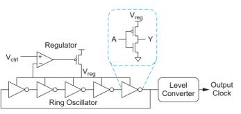
FIGURE 13.35 Voltage-controlled oscillator
