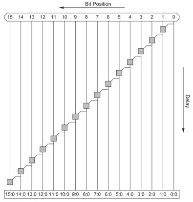
FIGURE 11.15 Carry-ripple adder group PG network
