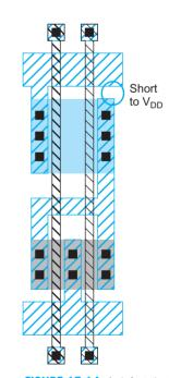
FIGURE 15.14 A defect that causes static *I*<sub>DD</sub> current
