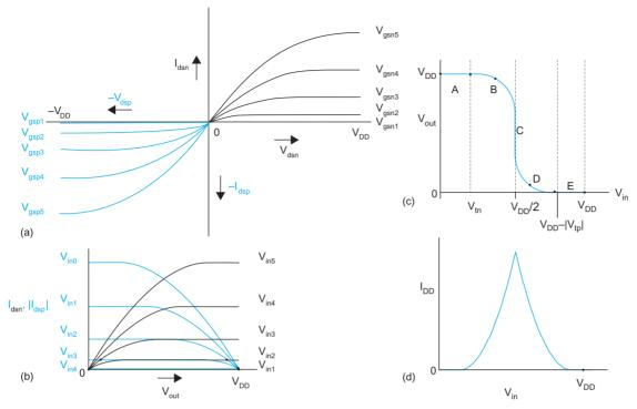
FIGURE 2.26 Graphical derivation of CMOS inverter DC characteristic
