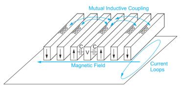
FIGURE 6.23 Inductive and capacitive crosstalk in a bus
