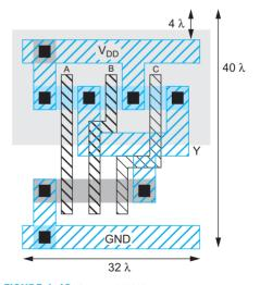
FIGURE 1.42 3-input NAND standard cell gate layouts
