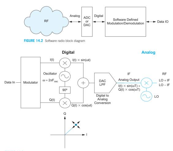
FIGURE 14.3 Software radio transmit path
