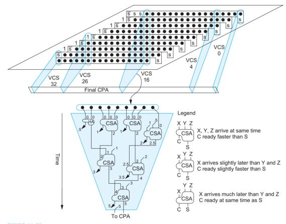
FIGURE 11.92 Vertical compressor slices in a TDM multiplier
