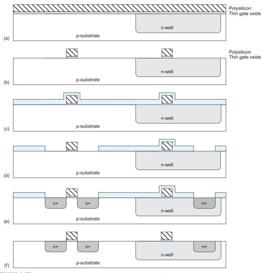
FIGURE 1.37 Cross-sections while manufacturing polysilicon and n-diffusion
