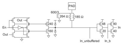
FIGURE 13.52 MOSIS bidirectional pad schematic
