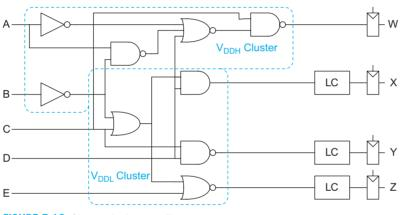
FIGURE 5.16 Clustered voltage scaling
