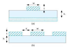
FIGURE 3.26 Microstrip and coplanar waveguide
