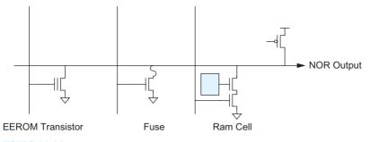
FIGURE 14.14 PLA NOR structure (one plane shown)
