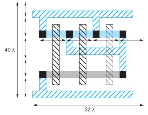
FIGURE 1.46 3-input NAND gate area estimation
