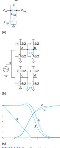
FIGURE 4.28 The effect of bootstrapping on inverter delay and waveform shape
