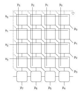
FIGURE 11.75 Rectangular array multiplier
