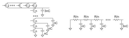
FIGURE 4.23 n-input NAND gate parasitic delay
