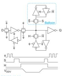
FIGURE 10.39 Balloon circuit for state retention
