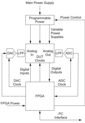
FIGURE 15.23 FPGA-assisted testing
