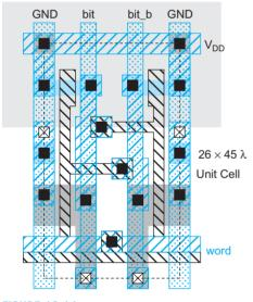
FIGURE 12.14 Layout of 6T SRAM cell. Color version on inside front cover.
