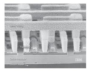
tor. Figure 9.62 shows a scanning electron micrograph of a 6-transistor static RAM cell in a 0.22  $\mu$ m IBM SOI process.
