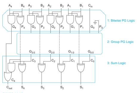
FIGURE 11.12 Addition with generate and propagate logic
