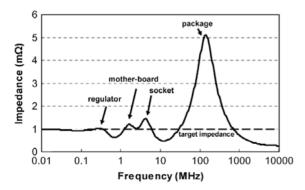
FIGURE 13.12 Pentium 4 simulated power supply impedance (© 2008 IEEE.)
