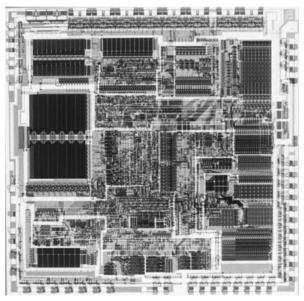
FIGURE 7.31 80286 microprocessor (Courtesy of Intel Corporation.)
