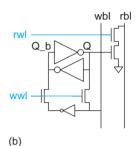
FIGURE 12.33 Register cell with single-ended write port
