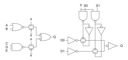
FIGURE 10.27 Combining logic and latches
