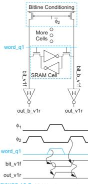
FIGURE 12.5 SRAM column read
