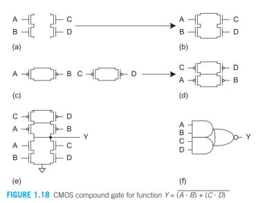
This AOI22 gate can be used as a 2-input inverting multiplexer by connecting  $C = \overline{A}$  as a select signal. Then,  $Y = \overline{B}$  if C is 0, while Y = D if C is 1. Section 1.4.8 shows a way to improve this multiplexer design.
