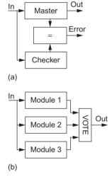
FIGURE 7.29 Master-checker operation and triple-mode redundancy
