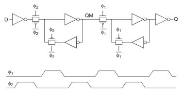
FIGURE 1.33 CMOS flip-flop with two-phase nonoverlapping clocks
