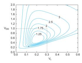
FIGURE 7.27 Contours of equal EDP accounting for variation, adapted from [Gonzalez97] (© IEEE 1997.)
