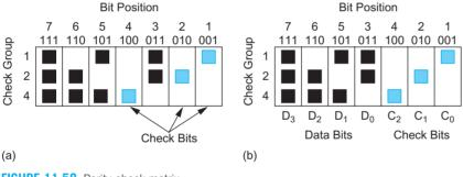
FIGURE 11.58 Parity-check matrix
