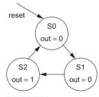
FIGURE A.33 Divide-by-3 counter state transition diagram
