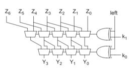
FIGURE 11.64 4-bit logarithmic funnel shifter
