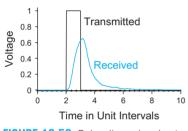
FIGURE 13.59 Pulse dispersion due to frequency-dependent attenuation
