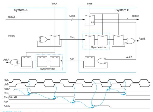
FIGURE 10.49 Two-phase handshake circuitry with synchronizers
