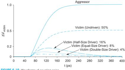
FIGURE 6.19 Waveforms of coupling noise
