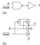
FIGURE 9.7 Resettable buffer optimized for data input
