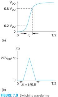
FIGURE 7.9 Switching waveform for RMS current estimation
