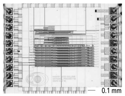
FIGURE 1.72 MIPS processor photomicrograph (only part of pad frame shown)
