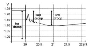
FIGURE 13.13 Pentium 4 simulated voltage droops (© 2006 IEEE.)
