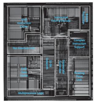
FIGURE 7.34 Pentium microprocessor (Courtesy of Intel Corporation.)
