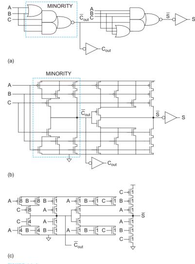
FIGURE 11.4 Full adder for carry-ripple operation
