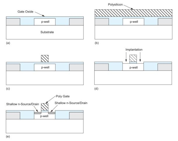
FIGURE 3.9 Gate and shallow source/drain definition
