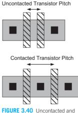
contacted transistor pitch
