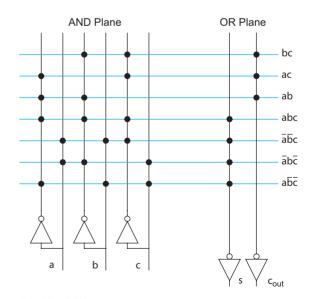
FIGURE 12.74 Dot diagram representation of PLA
