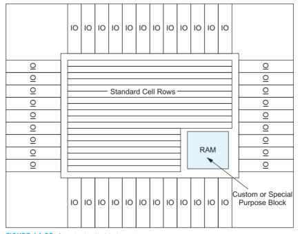
FIGURE 14.23 Standard cell chip layout
