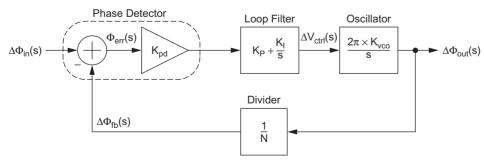
FIGURE 13.34 Linear system model of a PLL
