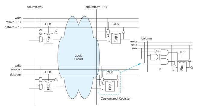
FIGURE 15.17 Parallel scan—basic structure
