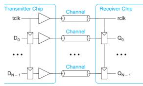
FIGURE 13.70 Source-synchronous system configuration
