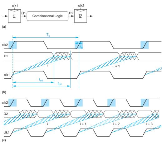
**FIGURE 10.52** Wave pipelining
