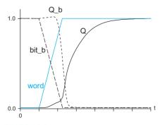
FIGURE 12.6 Write operation for 6T SRAM cell
