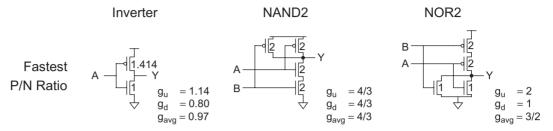
FIGURE 9.11 Gates with P/N ratios giving least delay
