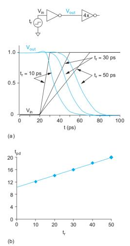
FIGURE 4.26 SPICE simulation of slope effect on CMOS inverter delay
