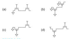
FIGURE 2.35 Pass transistor networks
