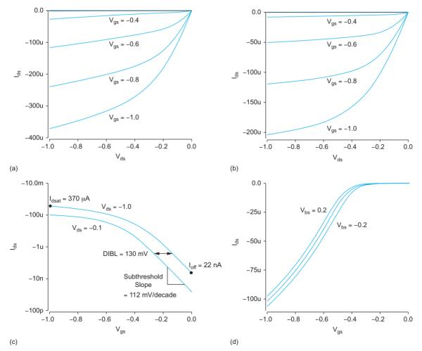
FIGURE 8.17 65 nm pMOS I-V characteristics
