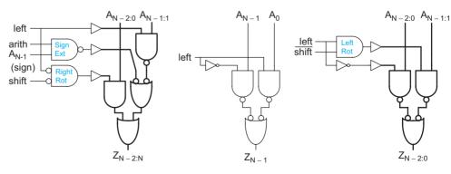
FIGURE 11.66 Optimized source generator logic
