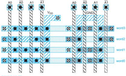
FIGURE 12.55 Row decoder layout on tight pitch
