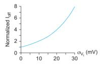
FIGURE 7.25 Impact of systematic threshold variation on worst-case leakage
