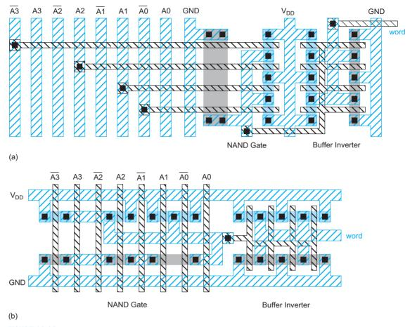
FIGURE 12.22 Stick diagrams of two decoder layouts
