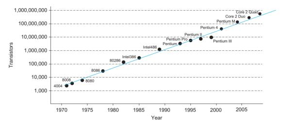
FIGURE 1.4 Transistors in Intel microprocessors [Intel10]
