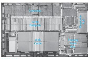
FIGURE 7.33 Intel486 microprocessor (Courtesy of Intel Corporation.)
