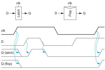
FIGURE 10.1 Latches and flip-flops
