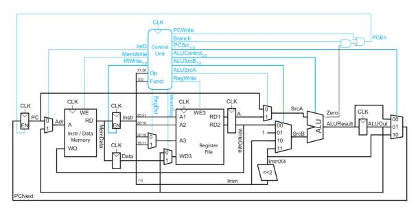
FIGURE 1.53 Multicycle MIPS microarchitecture. Adapted from [Patterson04] and [Harris07] with permission from Elsevier.
