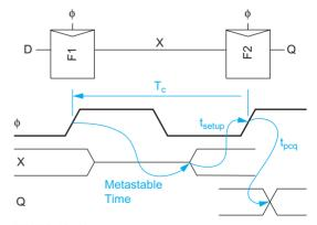
FIGURE 10.46 Simple synchronizer
