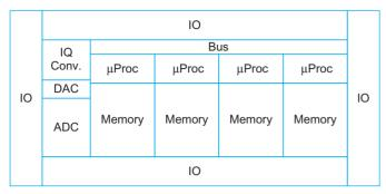
FIGURE 14.12 A possible floorplan for software radio
