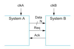
FIGURE 10.47 Communication between asynchronous systems
