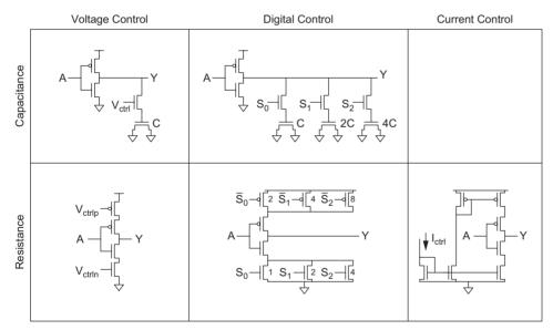
FIGURE 13.37 Alternative delay elements
