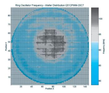
FIGURE 7.4 Wafer map of the frequency distribution of a ring oscillator circuit in 90-nm CMOS technology. From M. Pelgrom, "Nanometer CMOS: An Analog Design Challenge!" *IEEE Distinguished Lecture*, Denver 2006. (Figure courtesy of B. Ljevar (NXP). Reprinted with permission.)
