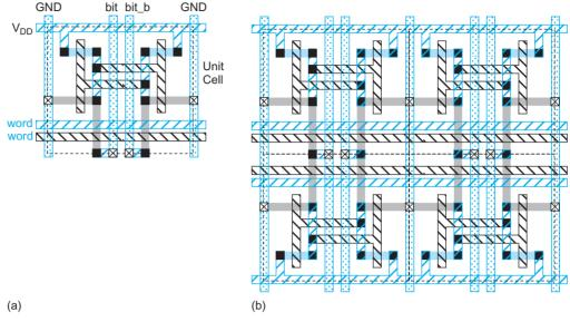
FIGURE 12.13 Stick diagram of 6T SRAM cell
