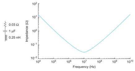
FIGURE 13.11 Impedance of bypass capacitor
