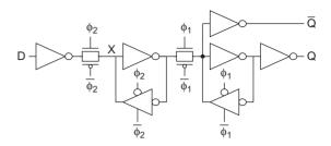
FIGURE 10.21 Flip-flop with two-phase nonoverlapping clocks
