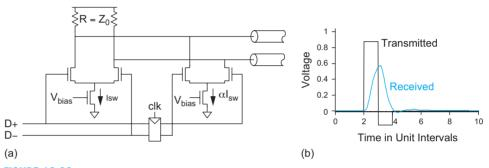
FIGURE 13.66 De-emphasizing transmitter (a) circuit, (b) de-emphasized pulses
