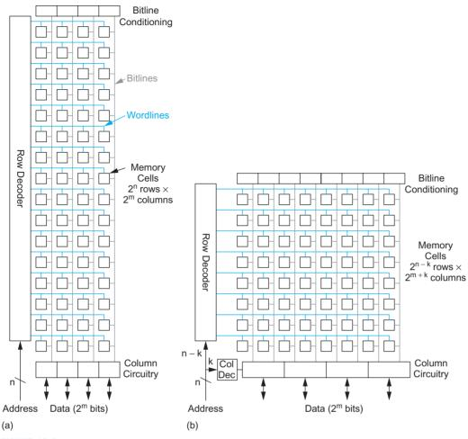
FIGURE 12.2 Memory array architecture
