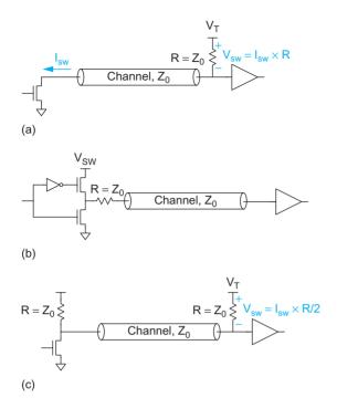
FIGURE 13.61 Transmission line drivers (a) current-mode driver (parallel termination at the receiving end), (b) voltage-mode driver (series termination at the transmitting end), (c) double-terminated driver (distinction between voltage and current is irrelevant)
