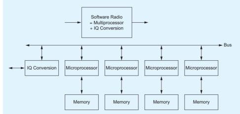
FIGURE 14.10 Software radio as a multiprocessor
