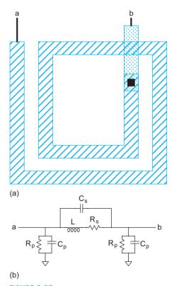
FIGURE 3.25 Typical spiral inductor and equivalent circuit [Rotella02]
