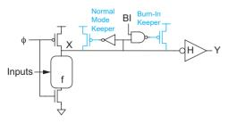
FIGURE 9.36 Burn-in conditional keeper
