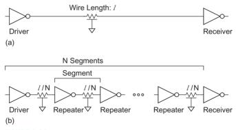
FIGURE 6.26 Wire with and without repeaters
