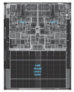
FIGURE 7.37 Core 2 Duo (Courtesy of Intel Corporation.)
