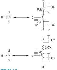
FIGURE 4.5 Equivalent circuits for transistors
