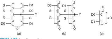
FIGURE 1.29 Inverting multiplexer
