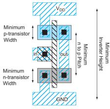
FIGURE 3.41 Minimum inverter height
