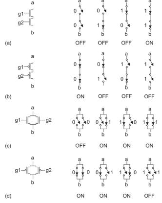
FIGURE 1.15 Connection and behavior of series and parallel transistors
