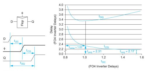
FIGURE 10.35 Flip-flop delay vs. data arrival time
