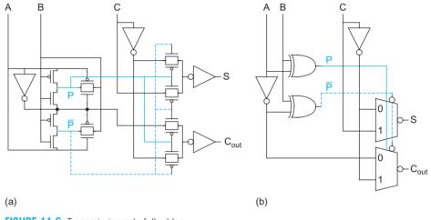
FIGURE 11.6 Transmission gate full adder
