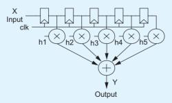
(b) Finite Impulse Response (FIR) Filter Structure
