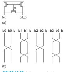
**FIGURE 12.29** Bitline noise reduction through equalizers and twisting
