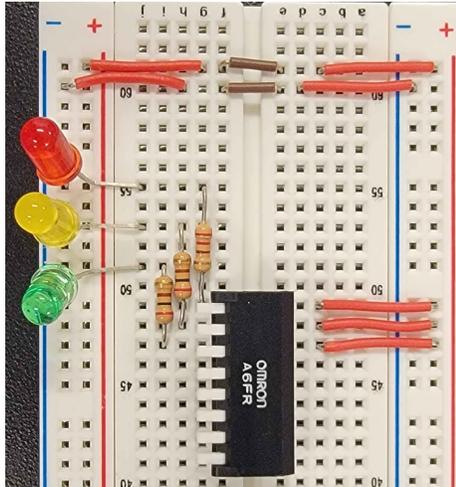
Switch 1 in “on” position; red LED on. This angle makes seeing the state of the switches easier.
