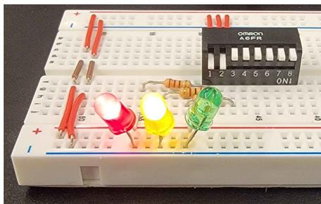
Switches 1, 2, and 3 in “on” position; red, yellow, and green LEDs on.
