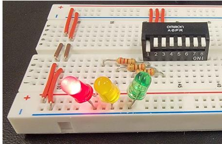
Switches 1 and 2 in “on” position; red and yellow LEDs on.
