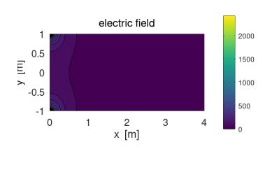
Fig. 3. Electric field strength between the plates
