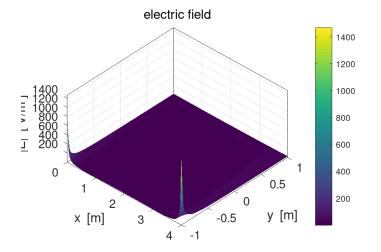
Fig. 8. The electric field inside a rectangle with non-constant boundary potential
