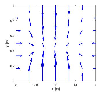
Fig. 4. Electric field inside the rectangle
