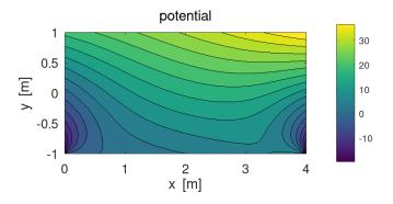
Fig. 9. The electric potential of a rectangle with non-constant potential
