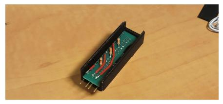
We had used a 20mil (~0.5mm) tolerance for the sliding fit (Galiki, Kondo, and Wilson 2023). The final fit was loose, but still acceptable. The fully assembled case with board inside is seen below:
