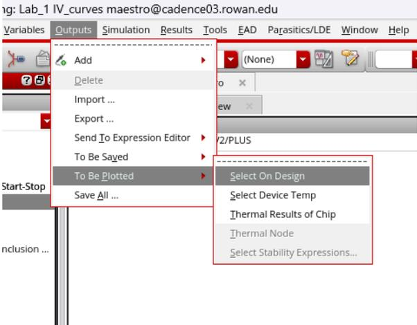
Outputs -> To be plotted -> select on design. (You can also type them in if you choose but keep in mind Cadence is case sensitive.) We want to measure the current on the drain of the NMOS with varying vgs. Please select the positive node of each of the 0v voltage sources connected to the drain of the NMOS.
