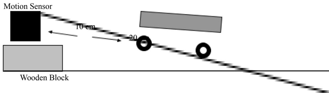
1. Make sure that the sensor is oriented such that it detects the cart and measures its position (i.e. distance from the sensor) all the way to the end of the track.
