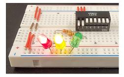
Switches 1, 2, and 3 in "on" position; red, yellow, and green LEDs on.
