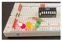
Switches 1 and 2 in "on" position; red and yellow LEDs on.
