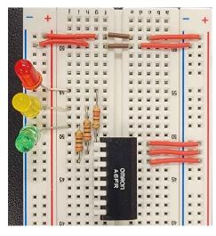
Switch 1 in "on" position; red LED on. This angle makes seeing the state of the switches easier.
