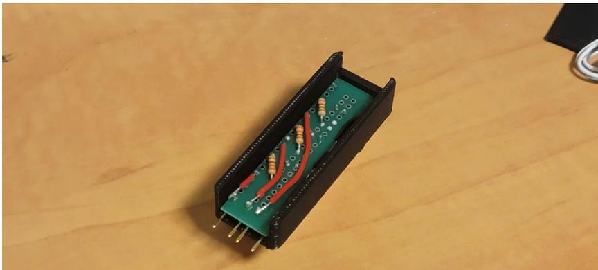
We had used a 20mil (~0.5mm) tolerance for the sliding fit (Galiki, Kondo, and Wilson 2023). The final fit was loose, but still acceptable. The fully assembled case with board inside is seen below:
