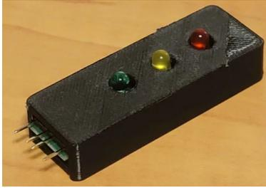
Plugging it in, we can confirm that the circuitry still works, and the pins are able to plug fully into the breadboard still, as seen below:
