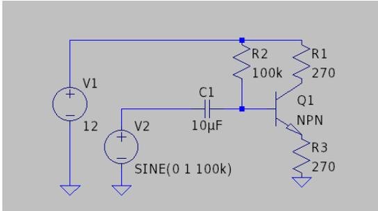
Fig. 3. Common Emitter Amplifier Schematic
