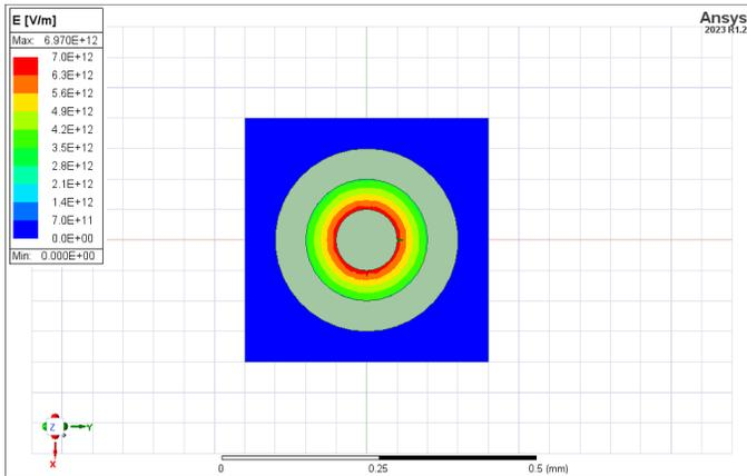
Fig. 4. Electric field between coaxial conductors
