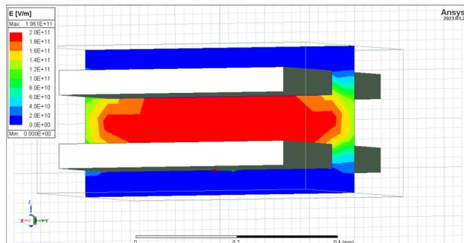
Fig. 2. Measuring electric field strength in the center of the capacitor
