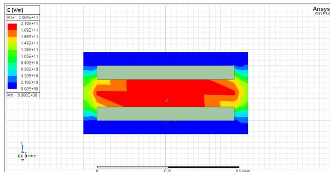
Fig. 1. Measuring electric field strength at the edge
