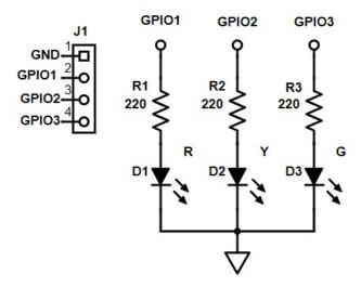
The goal of the completed board is to have a common ground pin and individual power pins for each LEDs. This allows for independent control of the LEDs. The components are all to be permanently affixed to the protoboard with solder. In doing so, our prototype will be more durable than a simple breadboard layout.
