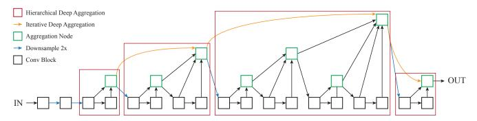
Figure 3: Deep layer aggregation learns to better extract the full spectrum of semantic and spatial information from a network. Iterative connections join neighboring stages to progressively deepen and spatially refine the representation. Hierarchical connections cross stages with trees that span the spectrum of layers to better propagate features and gradients.
